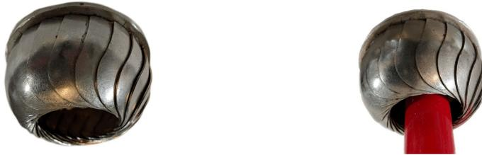
The first picture shows the CDS ABOP opened by the internal spring: it has 5 overlapping laser-cut blades just under 0.50" thickness, each, and together capable to withstand about 3000 PSI. More overlapping blades with higher thickness will proportionally increase the force the CDS ABOP can withhold. The shape of the CDS ABOP is in the form of a dome because it is the strongest possible architecture.
